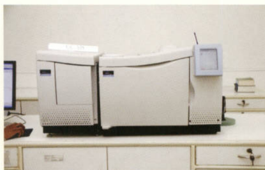
GC - MS : Gas Chromatograph Mass Spectrometer Identification of unknown volatile Compounds
