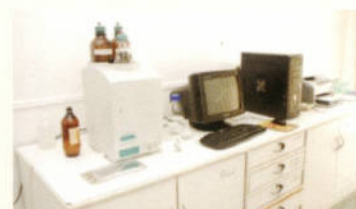
ION CHROMATOGRAPH Anion & Cation determination
