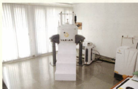
NMR - NUCLEAR MAGNETIC RESONANCE SPECTROMETER Organic Structure Determination H1, C13, P31, N14, F19, NMR
