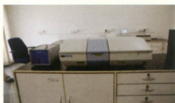
FTIR- Fourier Transform Infrared Spectrometer Functional Group Identification
