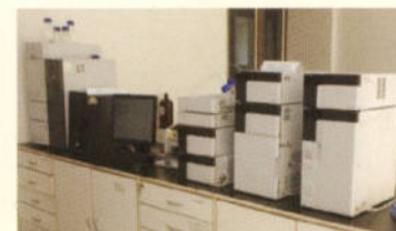
HPLC - High Performance Thin layer Chromatograph Purity determination of volatile Compounds
