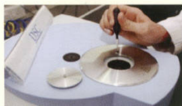
DSC - Differential Scanning Calorimeter To Study Various Polymer Properties
