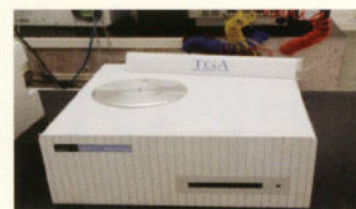
TGA - Thermo Gravimetric Analyzer To Study Various Chemical Reaction & Thermal Stability
