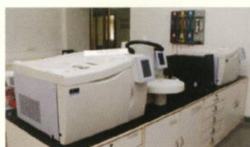
GC (ECD & NPD, FID & FPD DETECTOR) Purity Determination of Volatile Compounds
