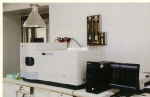
ICP - OES - Inductive Coupled Plasma Optical Emission Spectrometer Element Analysis in Soil, Water, Organic & Inorganic Material
